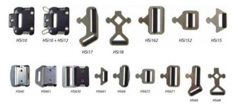
Charly Finsterwalder limits the lifetime of these buckles to 4 years when they are used on the paragliding harness **chest strap**. This means that all the harnesses with Charly Finsterwalder buckles on the **chest strap** that are older than 4 years can not be used any more. On the contrary, these CLICK-LOCK and T-Lock buckles maintain a lifetime of 10 years when they are used on the paragliding harness leg strap.
