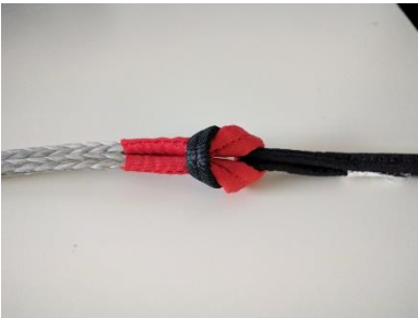
22. Connect the rescue and Y-bridle (supplied by harness manufacturer) by looping (larks foot). The connection must be centered in the field of the protection fabric (red).
