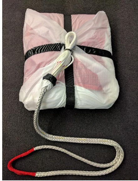
21. Close the 4 leaves of the rescue container with the last 50cm of lines.
